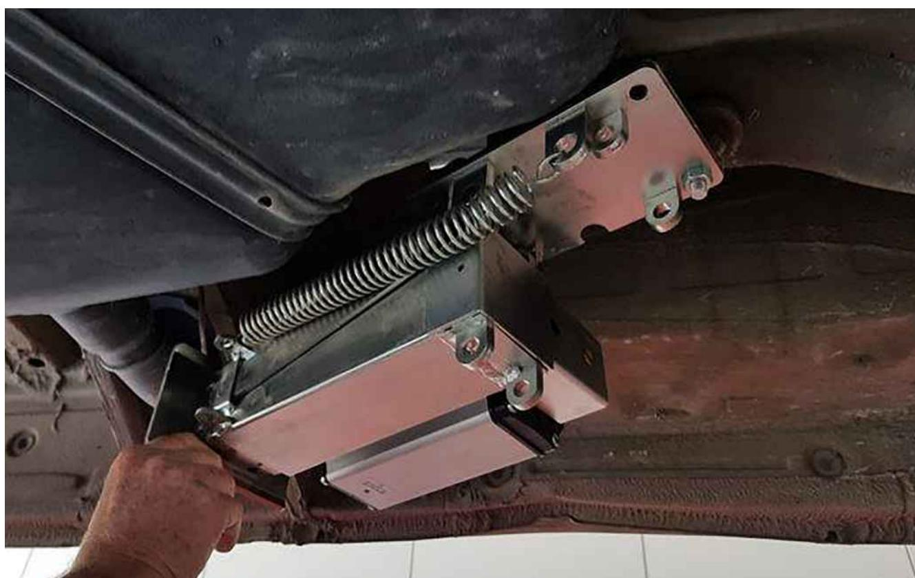
Motor jack facing towards the outside of the vehicle and rotation towards the rear
