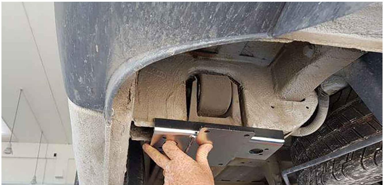
Put the adapter in the position shown in the photo, behind the support of the crossbow suspension.
