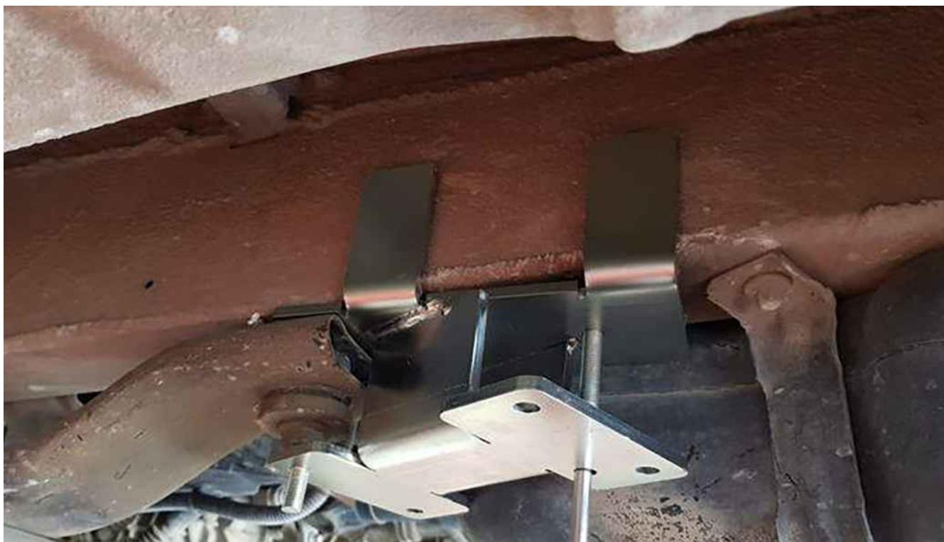
Fix the adapter with an M10 bolt.
